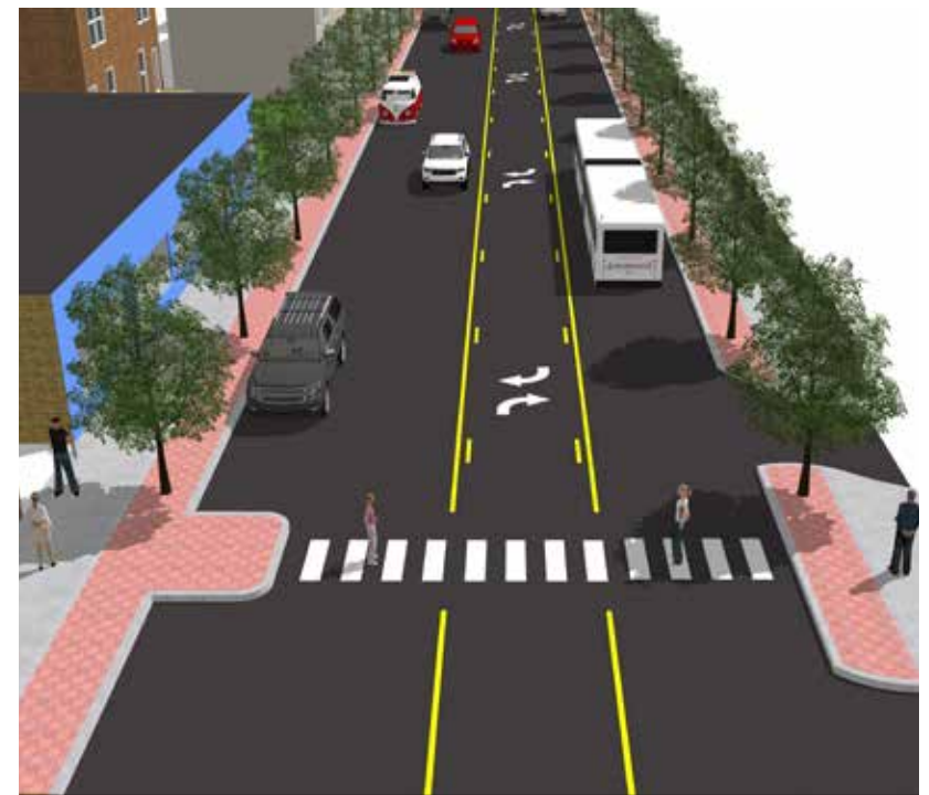
An example of a raised crosswalk and bumpout at the right-in, right-out across from Kroger
